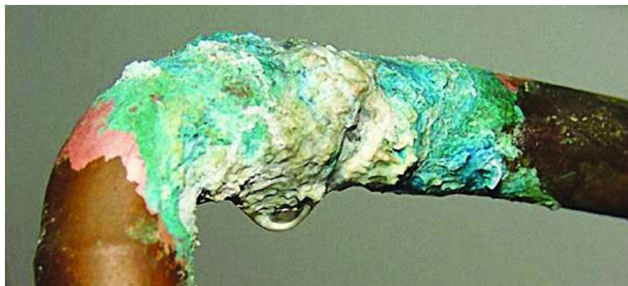
fig-17: Corrosion of copper
