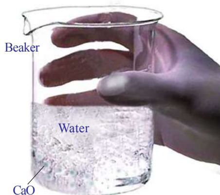
fig-5: Formation of slaked lime by the reaction of CaO with water
